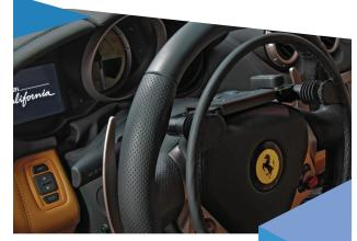
Wrapped in stylish Italian leather, the **Guidosimplex Over-Ring Electronic Accelerator** blends seamlessly with your vehicle's interior. Press on any point of the Ring to accelerate. Removal of the Over-Ring is quick and easy. The original functionality of the steering wheel airbag is retained. Pairs well with with Guidosimplex 907 Series brake levers.\*\*
