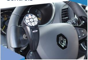
The Guidosimplex Stick-Steer is a compact, wireless, removable steering device with a built in keypad that allows fingertip operation of the vehicles secondary functions. Horn, Headlights, Turn Signals, and Wipers are all operated via a RF (Radio Frequency) connection. The keypad also features a backlight that can be set to match the vehicles interior lighting colors.
