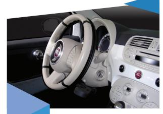
The unique design of the Guidosimplex Ghost Under-Ring Electronic Accelerator makes it almost invisible. Simply rotate the ring with your fingertips to accelerate. This Under-Ring design works well when there is limited space behind the steering wheel and requires very little effort to accelerate.\*\*
