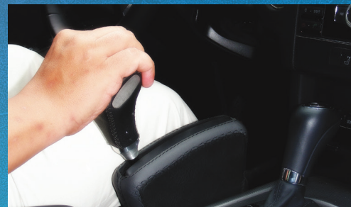
F1 EVO Accelerator/Brake Floor Mount Mechanical pull for acceleration and push for brake
