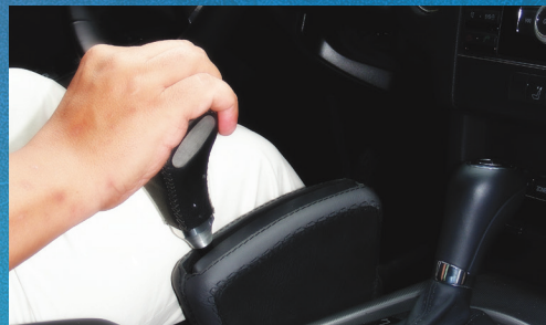
F1 EVO Accelerator/Brake Floor Mount Mechanical pull for acceleration and push for brake
